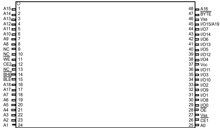
Figure 5. 48-pin TSOP I Pinout (with ERR (Top View)) [3, 4]
