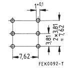
Hole arrangement View in mounting direction
