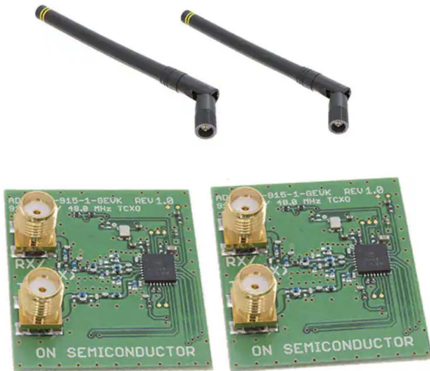
Figure 2. Content of the ADD5043-915-x-GEVK Kit
