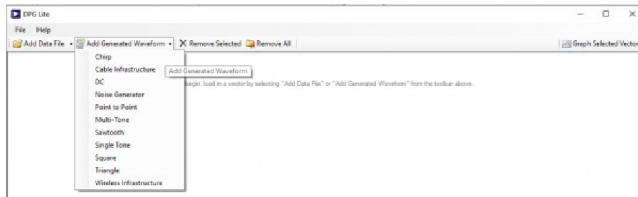
Figure 21a. Waveforms that can be generated using DPG Lite
