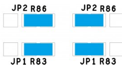
Figure 14a. DAC clock is connected to on-board oscillator (default) | Figure 14b. DAC clock is connected to J10
