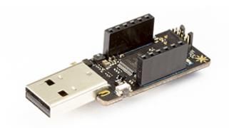
The Particle Debugger gives you the power of professional debugging at a fraction of the cost. Using this accessory, you'll be able to program Particle Gen 3 hardware over common interfaces like JTAG and SWD, using open source tools like GDB and openocd. It can also be used with Gen 2 devices, with the addition of some jumper wires.
