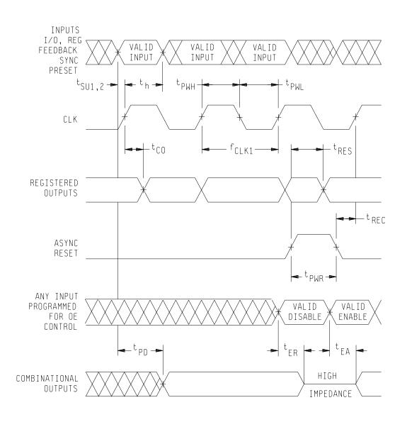
FIGURE 4. Switching waveforms.
