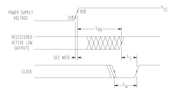
Note: The power-up reset feature ensures that all flip-flops will be reset to low after the device has been powered up. The following conditions are required:
