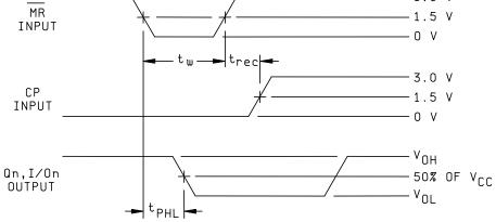
FIGURE 5. Switching waveforms and test circuit.
