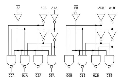
FIGURE 3. Logic diagram.
