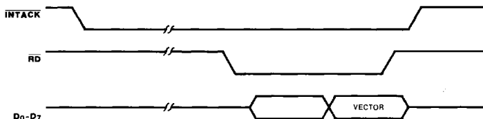
Figure 14. Interrupt Acknowledge Cycle Timing
