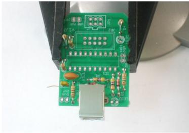
When you solder in the parts, make sure that you put plenty of solder on the two prongs that hold the USB connector in.
