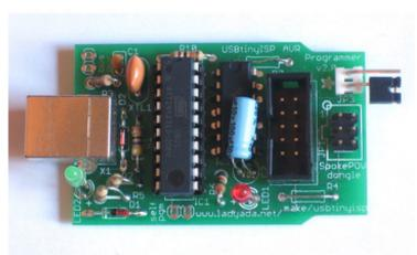
do the remaining 5 all at once. Place **R10** (10K pullup resistor), **R3**, **R5** and **R6** (1.5K resistors for the USB connection, LEDs and output buffer).
