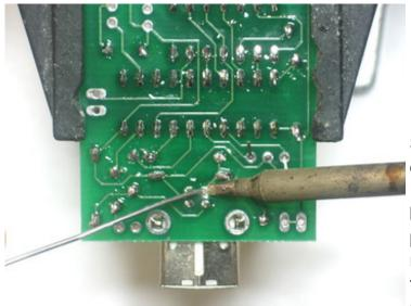
Solder in the three-pins of the oscillator and all 6 pins of the USB connector. Make sure to not bridge any of the square-pins and put plenty of solder on the mechanical tabs. These provide the resistance when you plug in a cable so it's important that they are soldered well, as shown here.
