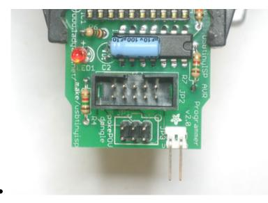
Almost done! The last set of parts are the headers for the cables, and the jumper header. The 10-pin box header has a notch in it, make sure it matches up with the silkscreen, as shown.
