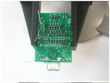
In this image, the negative side for the green LED is on the left. The negative side for the red LED is towards the top.
