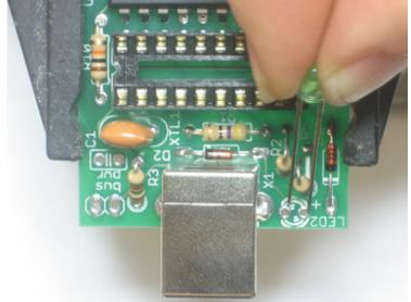
Next are the two indicator LEDs, green **LED2** and red **LED1**. These LEDs let you know that the USB device connected successfully, and is in the process of programming the target device.
