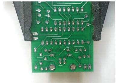
When you are done, it should look like this. If you have some sticky stuff on the solder joints, that's OK, that's the rosin inside the solder that protects the joints from oxidation. It isn't necessary to clean it off.
