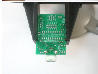
Next are the headers and the microcontroller socket. The 6-pin header has no direction so just put it in either way.
