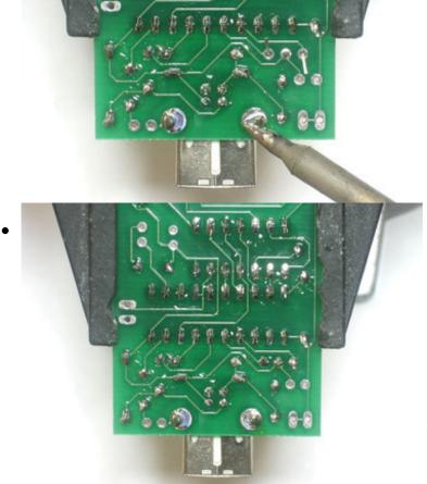
Although they are short, you should clip the pins to the oscillator if possible, to make sure they dont bend over and touch another component.
