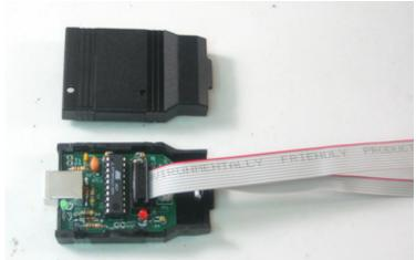
Plug in the two cables as shown, the red stripes on top and so that the cables don't bend over the plug (the case wont fit).
