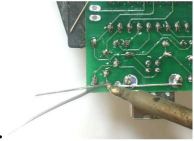
Solder and clip the two LEDs.
