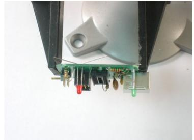
Place the LEDs as shown, the red one near the 10-pin header and the green one near the USB plug.
