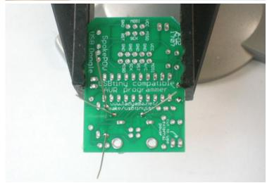
Next up are the 2 47 ohm resistors. Place them as shown. Bend the legs out, flip the PCB, solder the 4 joints and clip them.
