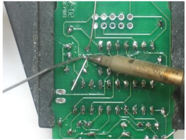
Solder and clip both capacitor's leads.
