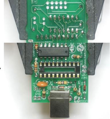
Next is the USB connector and the 12.00MHz ceramic oscillator. The USB connector is what we use to plug into the computer, the oscillator makes sure the USBtiny microcontroller runs at the precise rate necessary to communicate at the very picky USB protocol rates.
