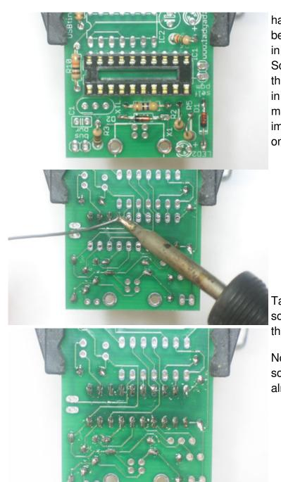
hard work. A socket is useful because you can replace the chip in case of upgrade or damage. Sockets have a little notch in them to indicate which way to put in the chip. This notch should match the notch in the silkscreen image, in this picture, the notch is on the left-hand side.
