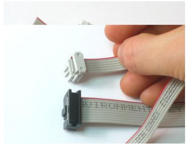
It's important that the key (the bump in the connector) and the red stripe line up. Match the image on the left, just poke the conductor in with a mm or two past the edge.
