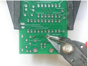
Next, clip the excess leads using the diagonal cutters. Clip right above the top of the solder joint.
