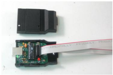
Put the PCB into the bottom case half.
