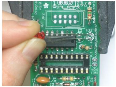
LEDs are diodes, and must be placed correctly or they wont light up, which is very confusing.
