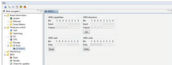
Figure 11: Configuring GPIO Pins using JIDA32/K-Station
