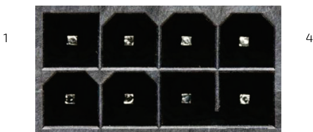
Figure 17: ATX Power connector with 8 pins
