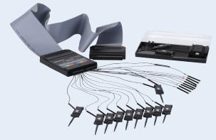
The 16-channel color-coded logic probe consists of two eight-channel pods. To make contact with the DUT, the probe connects directly to square pins or clips to test points using the included grabbers. With an input capacitance of only 8 pF and 100  $k\Omega$  input impedance, the probe protects the integrity of your signal. The probe is included with MSO models.
