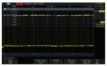
Select up to 2 serial bus protocols I<sup>2</sup>C, SPI, UART/RS232, CAN, and LIN and decode concurrently from analog and MSO channels. Decode information in real-time and display in binary, decimal, hex, or ASCII.
