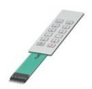
Membrane keypad, self-adhesive, silver conduction technology, 12 keys, embossed, 3 colors, connecting cable: 88.5 mm, with crimp female connector, pitch: 2.54 mm, operating temperature: -20°C ... 70°C
