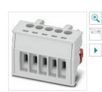
PCB connector, nominal cross section: 1.5 mm², color: light gray, rated voltage (III/2): 150 V, contact surface: Tin, type of contact: Female connector, Number of potentials: 5, Number of rows: 1, Number of positions per row: 5, number of connections: 5, product range: ICC..-PSC1,5/..-3,5, pitch: 3.5 mm, connection method: Screw connection with tension sleeve, conductor/PCB connection direction: 0 °, Locking clip: - Locking clip, Locking: without, type of packaging: packed in cardboard
